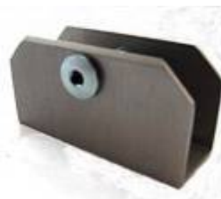
PH12 DOOR HING FOR 18mm TO 20mm BOARD, BOLT THROUGH FACIA SCREW FIX OR BOLT THROUGH WITH NYLON RISERS
